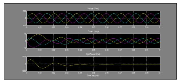
Fig.8 Waveform showing stator voltage, stator current and power flow capability
