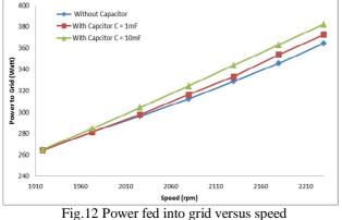
Fig.12 Fower led into grid versus spe
