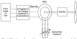
Fig. 4 Circuit topology of the combined input voltage and slip power control scheme
