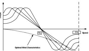
Fig. 3 Characteristics of a WRIG with rotor resistance control
