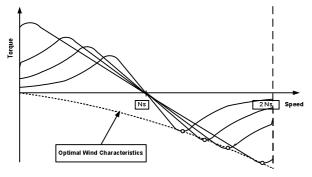
Fig. 5 Characteristics of a WRIG with rotor resistance as well as stator voltage control
