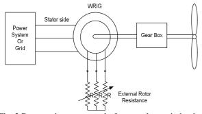
Fig. 2 Rotor resistance control of a wound rotor induction generator
