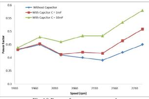
Fig.10 Power factor versus speed
